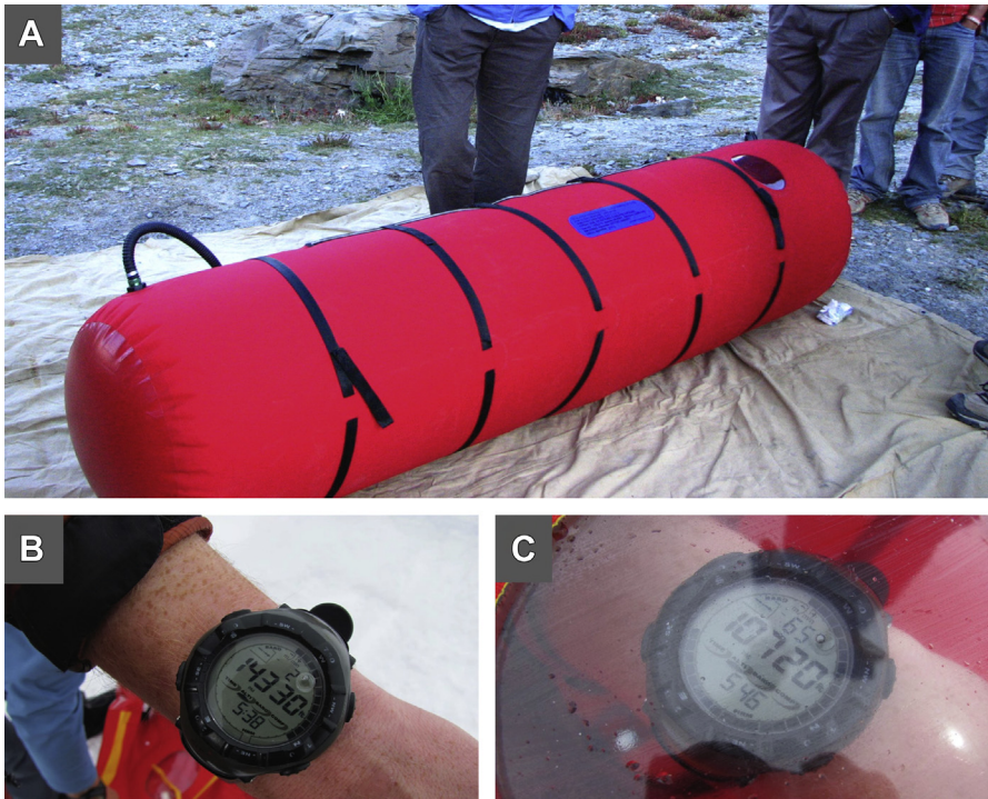
Fig. 1. Portable hyperbaric chamber. (A) Once an ill individual is placed inside the bag, a tight-fitting zipper is closed and the bag is inflated using a foot pump. Barometric pressure rises inside the bag, simulating a descent in altitude, as shown in the photo of an individual holding an altimeter watch outside (B) and inside (C) the bag following inflation. The magnitude of simulated descent varies based on the altitude of use and inflation pressure. Continuous pumping is required after initial inflation to maintain pressure and ensure adequate ventilation.
