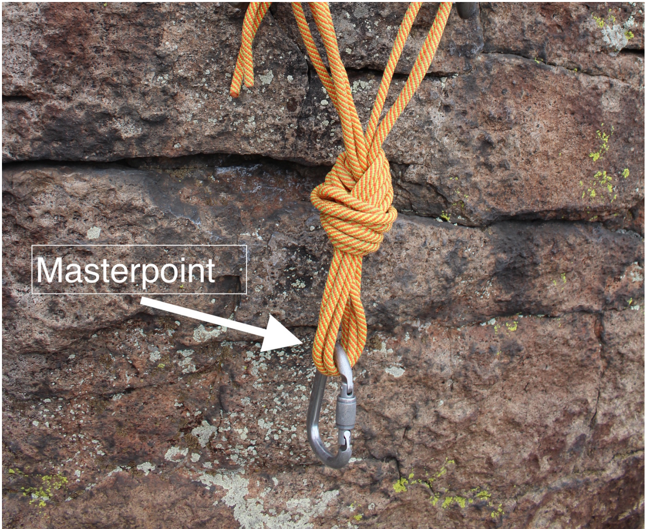
Similarly, a simple ponytail anchor with a cordellette provides a masterpoint with the effective strength of four strands of 7mm nylon cord.
