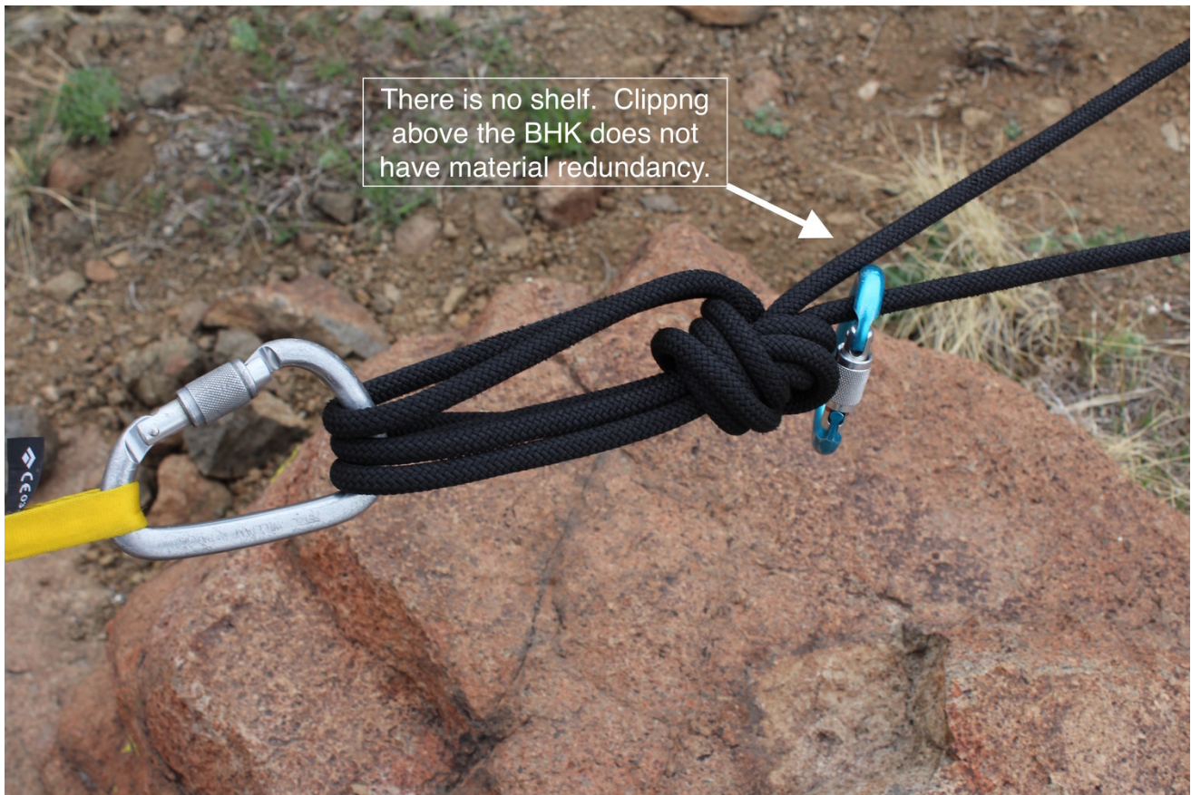
Looking closer, it is clear that clipping above the BHK on this anchor does not have the same material redundancy as the BHK itself.
