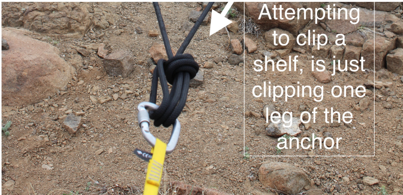
Many Toprope anchors that are built with a static rope effectively do not have a shelf.
