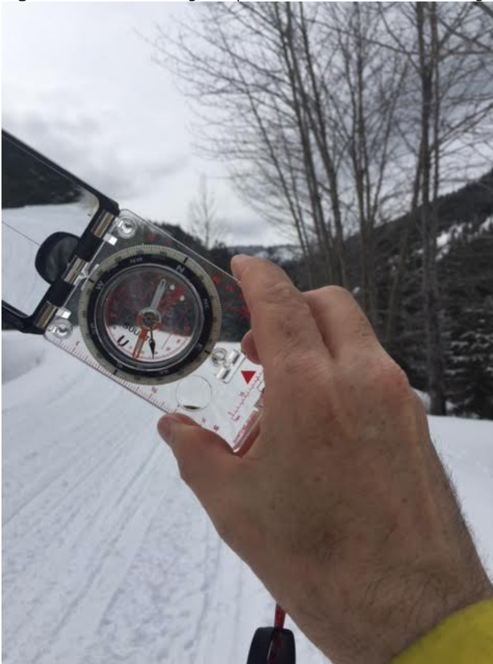
Figure 3. Hand bearing compass inclinometer reads 36 degrees.
