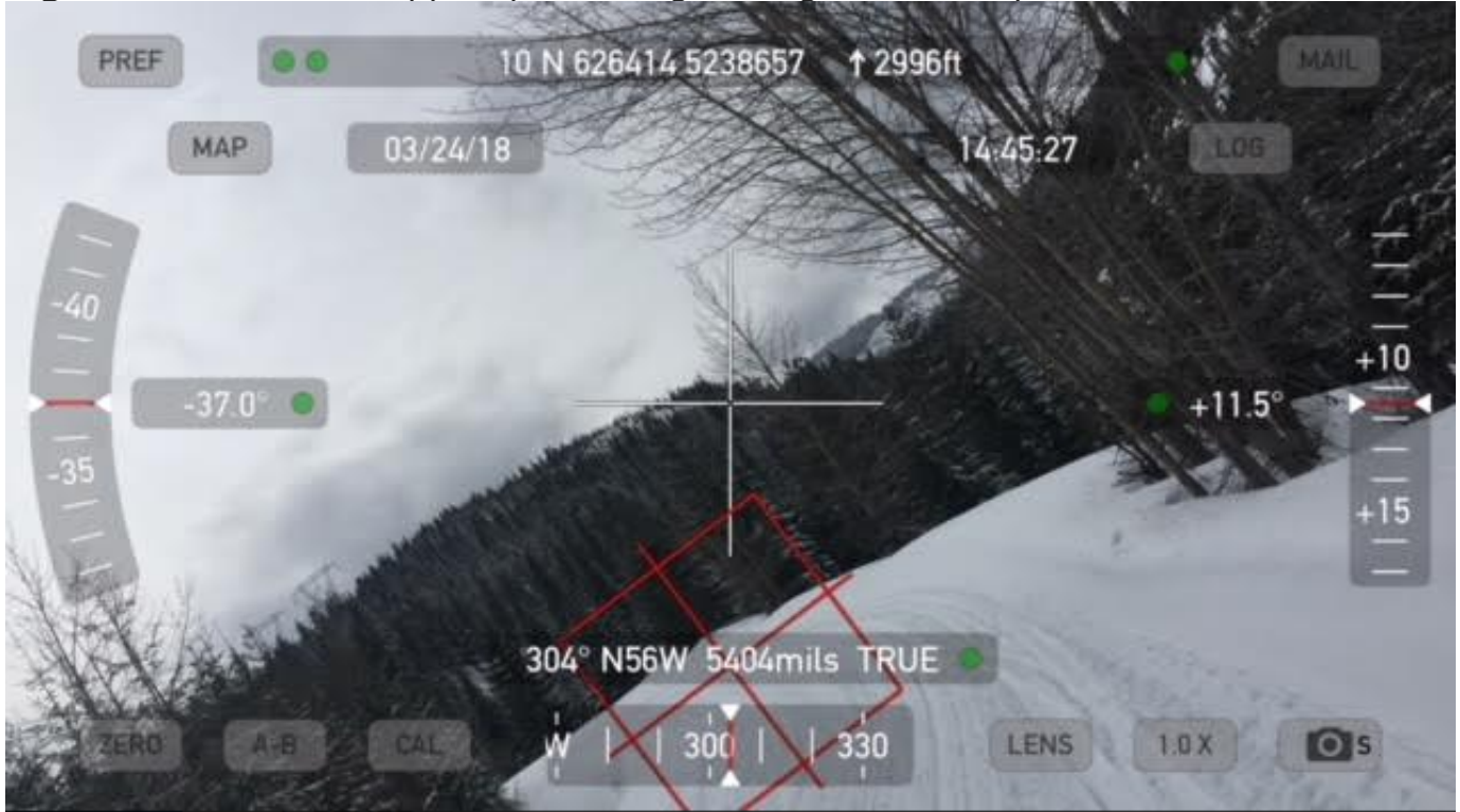
Figure 2. Theodolite app slope reading 37 degrees in left panel.
